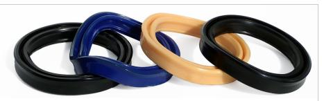
Polyurethanes are a thermoplastic elastomer. High heat causes the material to soften. High heat melt sample of Resilon 4350 seals (black), Resilon 4300 seal (tan), Leading competitor seal (blue) shown above.
