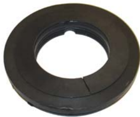
Failed Seal Resulting from Improper Fit
