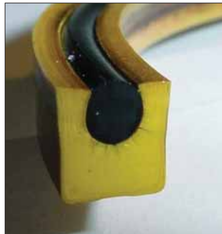
Figure 2-9. Seal exhibiting nearly 100% compression set
