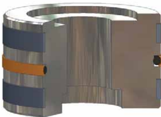
CP installed in Piston Gland
