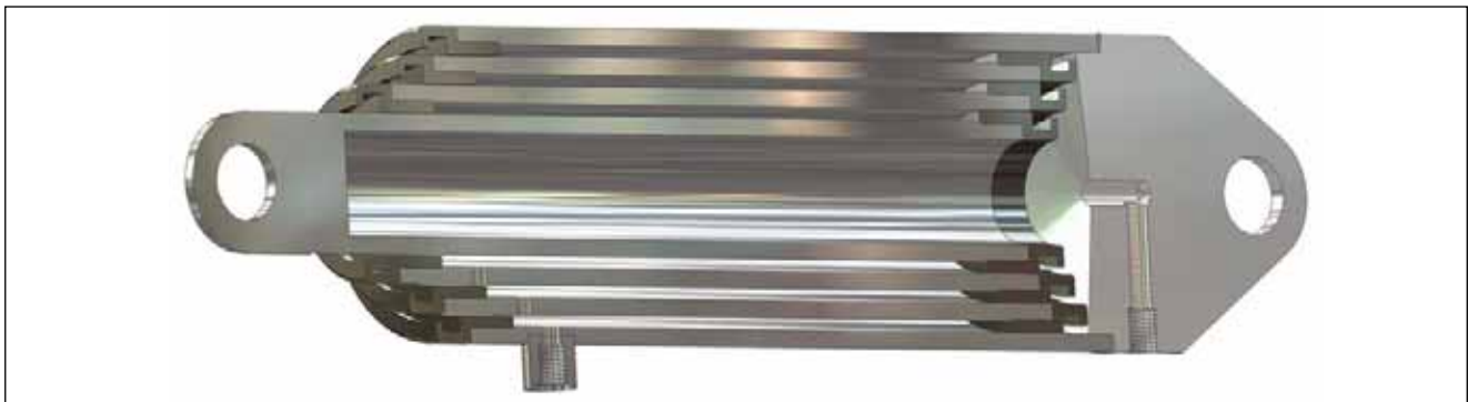
Figure 4-5. Telescoping Power Cylinder
