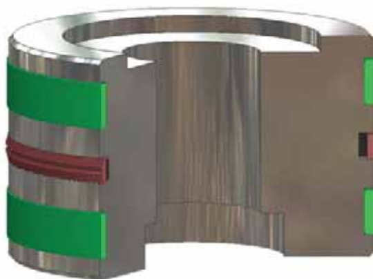
BP installed in Piston Gland
