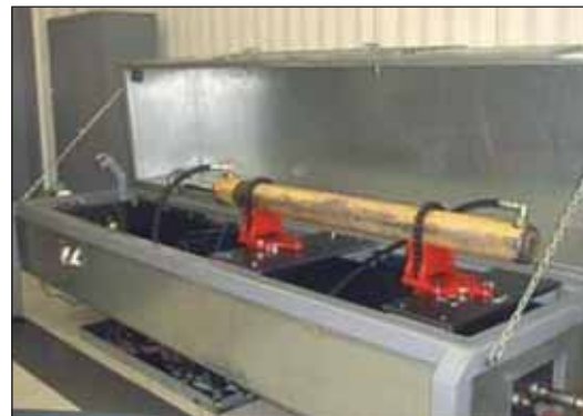
High pressure hydraulic leakage testing
