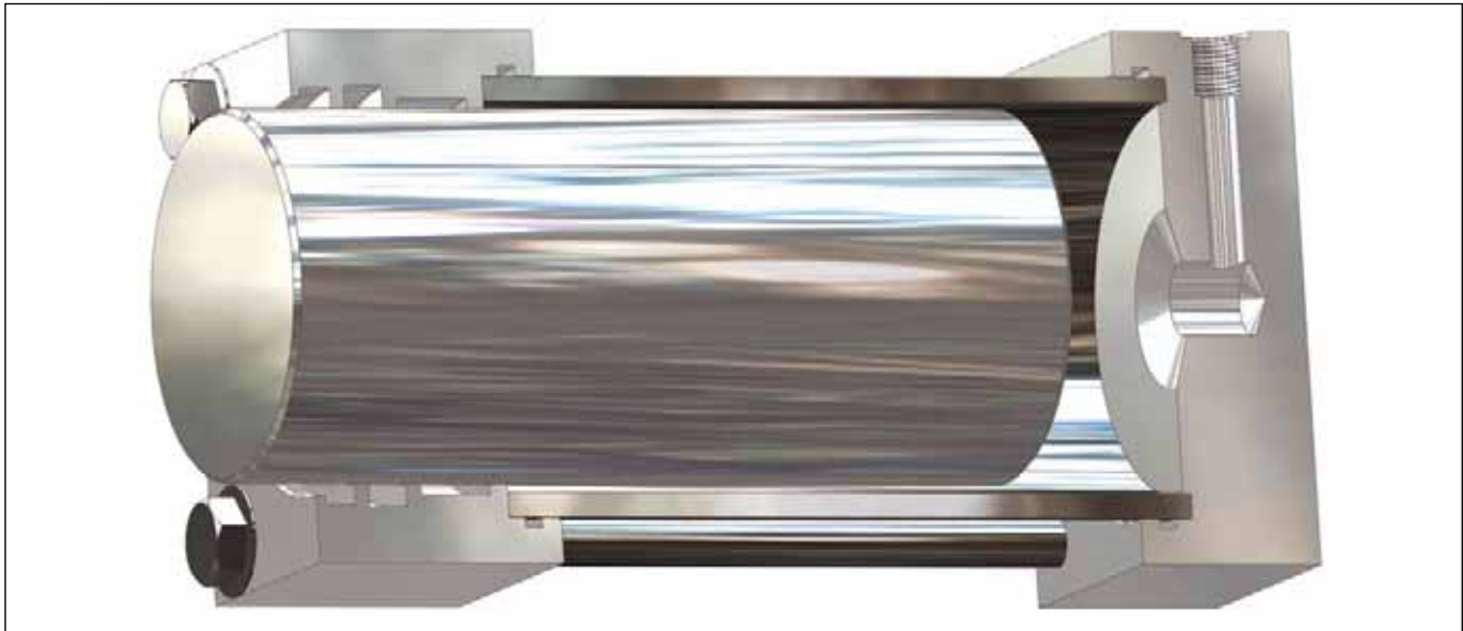
Figure 4-2. Single Acting Hydraulic Ram
